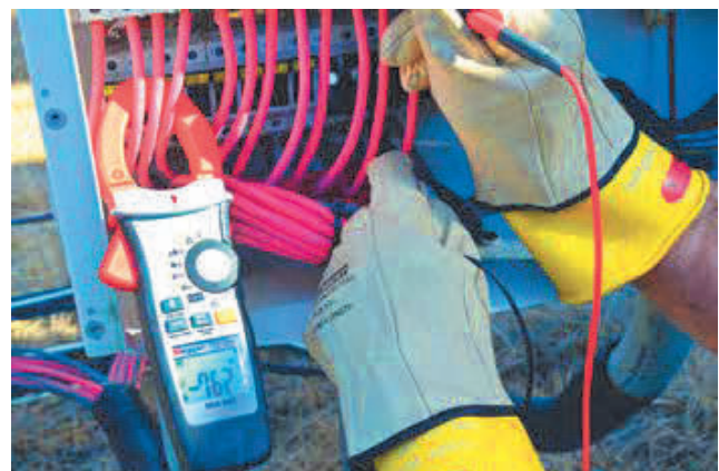
Figure 4-6: When meter leads are reversed, a negative sign of the same voltage value verifies proper polarity in each circuit. If a negative voltage is measured with the leads in the correct position, this indicates that the PV string was connected incorrectly during installation.
