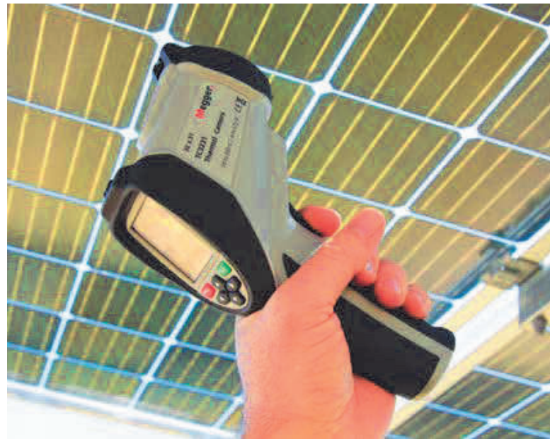
Figure 4-21: PV module temperature is measured by making direct contact with the backside of the module under test. A thermal camera may be used, or a temperature sensor that integrates with the technician's DMM as is shown in Figure 4-8.
