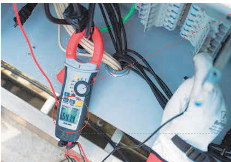
Figure 4-23: Verify correct polarity by swapping the lead locations and re-measuring voltage. The DMM should display the same voltage as the initial reading but with a negative sign.
