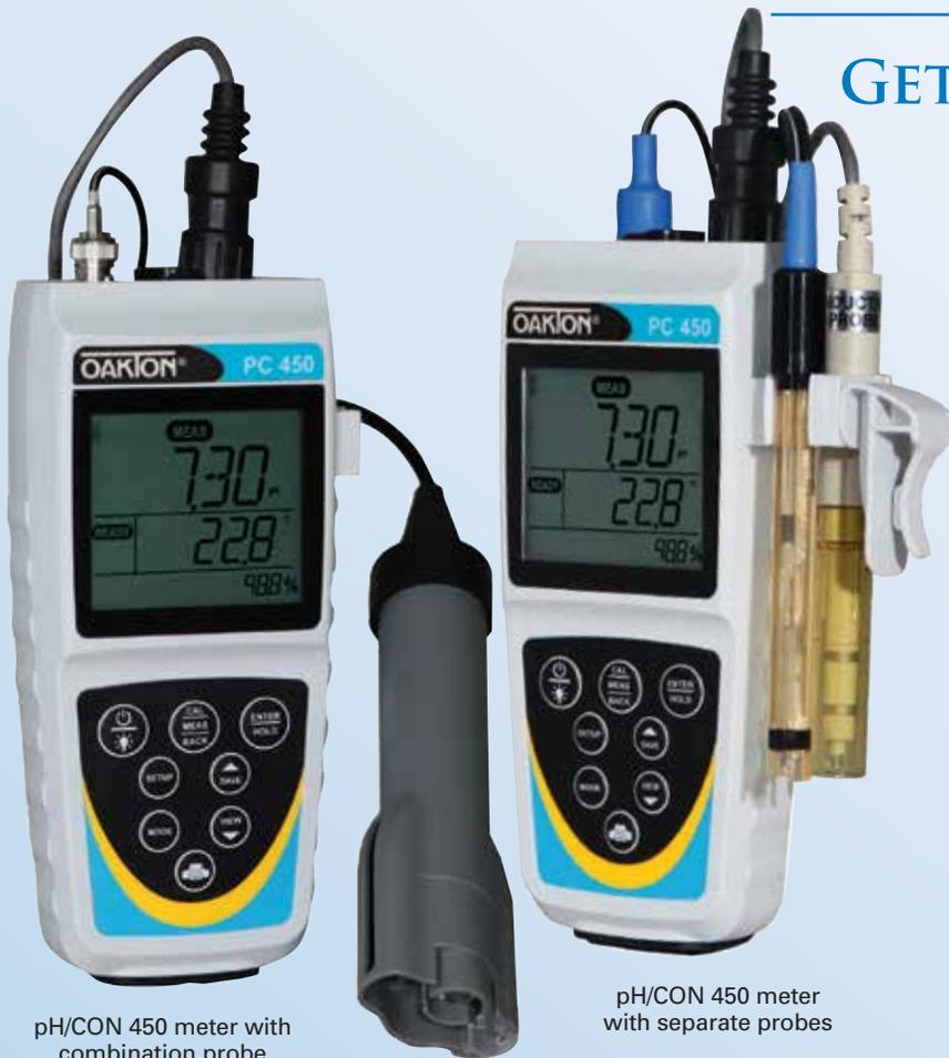
pH/CON 450 meter with combination probe
