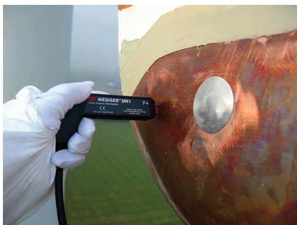
Figure 7: Lightning Conductor Resistance Measurement at Blade Tip
