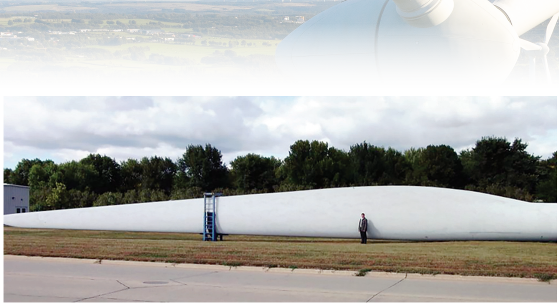
Figure 9: Wind Turbine Blade before Installation
