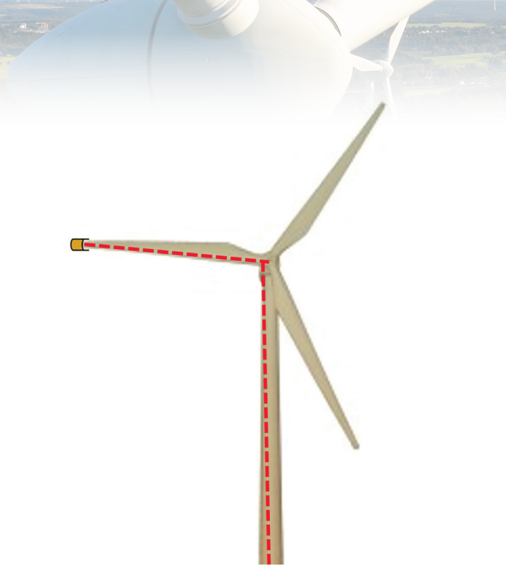
Figure 4: Current Path for Lightning Discharges
