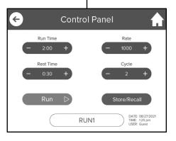
On the Control Panel, runtime parameters can be set as well as stored or recalled.
