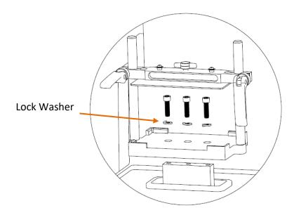
Figure 1 – Installing the Clamp
