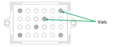
Figure 4 – Top view of Clamp with 2 mL Vials in Corner and Center Positions
