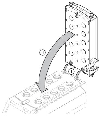
**Step 2**Lock the Manifold in position by pulling the latch on the Integrity to engage the front foot.
