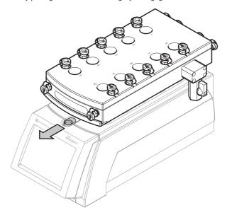
Connect the gas feeds to left and/or right hand gas inlets on the rear of the Manifold as required. Ensure the release button is in the UP position, if the release button is in the DOWN position press the release button. To use a single gas feed, connect the gas supply to the left hand inlet on the rear of the unit and link the left hand outlet on the front to the right hand inlet on the front. The gas will then exit via the gas management module on the right hand side of the unit.
