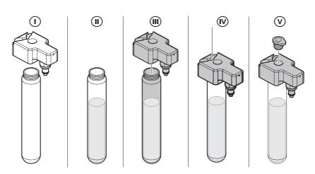
Position the tube/cap assembly in the appropriate well and push down until the fitting clicks to engage the gas supply.
