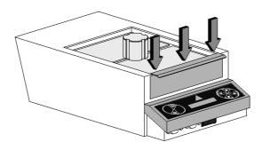
Carefully slide the Reaction Block into position ensuring the central screw of the reactor block is located firmly into the slot provided on the slide plate.
