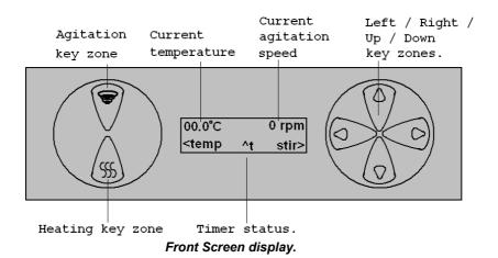
Touch the left hand illuminated key zone from the group of four key zones on the control panel to move into temperature selection mode. The direction is indicated by the (<) symbol next to the word 'temp' on the display.
