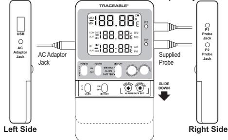
labeled "P1" and probe labeled P2 must be plugged into the probe jack labeled "P2".
