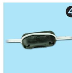
This completes the installation of the suppressor.
