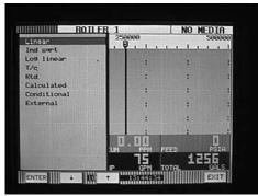
7. The menu displaying types of linear inputs should now appear. (Selections may appear different from the screen example to the left.) For this example use the up/down arrow keys to select the 12.5V (for 12.5 Volt) range then touch ENTER.
