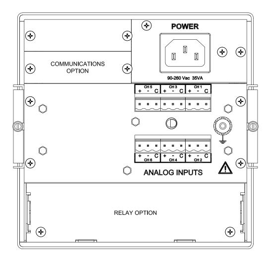
Figure 2-6 DC2000 Rear Panel Connections
