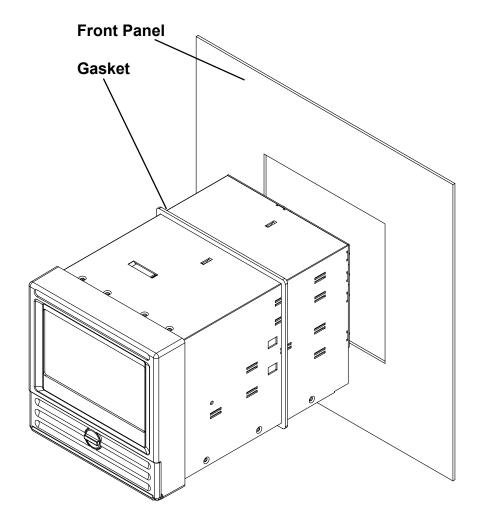
**Figure 2-2 Front Panel Insertion**
