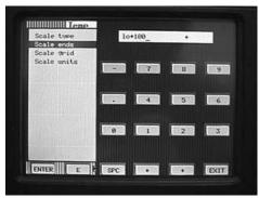
18. You will now be prompted with mid→ ←. To illustrate one of the features of the Recorder we will enter a value that is not 50% of the desired range. For this example, enter 200 and touch ENTER. The result will be two linear ranges. One will have high resolution and the other will have low resolution.
