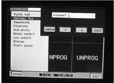
11. You will now be back at the menu starting with **Point tag**. Use the up/down arrow keys to select **Basepoint** and touch **ENTER**. You will be prompted with **base pt?**. Use the up/down arrow keys to select the channel from which the totalizer will derive its information. For this example, select channel 1 and touch **ENTER**.
