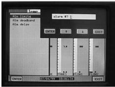
17. The alarm types menu will now be displayed. Using the up/down arrow keys you can select the type of alarm you wish to configure. For this example we want to know when the flow exceeds 120 gpm. Select Type=high and touch ENTER.
