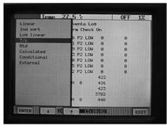
7. The menu displaying thermocouple types should now appear. For this example use the up/down arrow keys to select **J t/c** and then touch **ENTER**.
