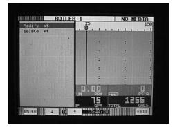
6. The menu containing types of inputs should now be displayed. Use the up/down arrow keys to select **Linear** and then touch **ENTER**.
