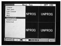
7. The menu displaying the various calculated channel types should now appear. For this example use the up/down arrow keys to select **Totalize** and then touch **ENTER**.
