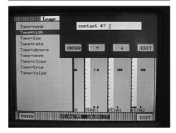
Touch EXIT twice to get back to the menu beginning with Point tag. Using the up/down arrow keys select Chart scale and touch ENTER. Using the up/down arrows you can select A, B, C, D, E, F, G or H. For this example select A and touch ENTER.
