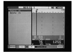
The menu containing types of inputs should now be displayed. Use the up/down arrow keys to select Linear then touch ENTER.
