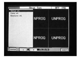
The menu containing types of inputs should now be displayed. Use the up/down arrow keys to select Calculated and then touch ENTER.
