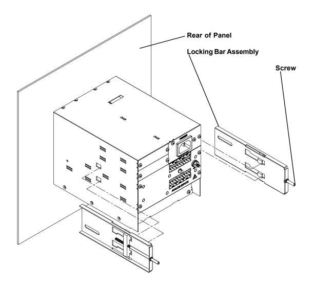
Figure 2-3 Rear View Panel Installation
