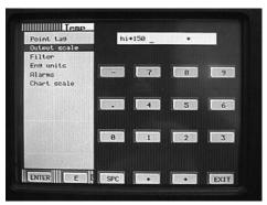
13. Using the up/down arrow keys select Eng units and touch ENTER. An alpha-numeric keypad will appear prompting you units→ ←. You can enter up to 5 characters. Using the PAGE, PAGBK and SHIFT keys, if needed, enter the desired engineering units. For this application enter GPM and touch ENTER.
