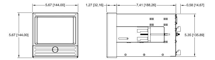
Figure 2-1 Recorder Dimensions in Inches [mm]
