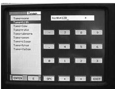
19. You will next be prompted **contact #?**. If your recorder is fitted with alarm contact outputs, you can select which contact will change state when the internal high alarm activates. Using the up/down arrows you can select 0, 1, 2, 3, 4, 5 or 6. For this example select 2 and touch **ENTER**.
