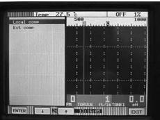
12. You should now be back at the Point tag menu. Use the up/down arrow keys to select Eng units and touch ENTER. You will be prompted with units (°C or °F). For this example use the up/down arrow keys to select °C and touch ENTER.
