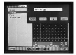
16. You will now be in the scale menu. Use the up/down arrow keys to select **Scale ends** and touch **ENTER**. You will be prompted with **places?** (for decimal places). Using the up/down arrow keys you can select 0, 1, 2, 3, 4 or 5. For thermocouples you would only select 0 or 1. For this example select 1 and touch **ENTER**.
