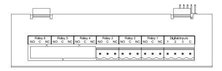
Figure 2-8 Mechanical Relay Connections (3 Channel Shown)
