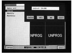
20. You will now be back at the Reset Control menu. Use the up/down arrow keys to select Reset print and touch ENTER. You will be prompted with print=NO\*. Touch the YES key then touch ENTER. This enables the Recorder to post the totalizer reset information to the alarm/event page which is where you would view your daily totals.
