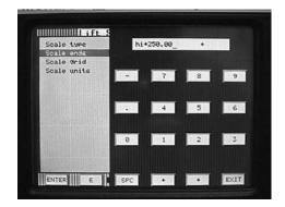
26. You will now be back at the scale setup menu. Use the up/down arrow keys to select Scale units and touch ENTER. The alphanumeric keypad will be displayed. This is what will be displayed as engineering units in the trend mode only. For this example enter PSIG and touch ENTER.
