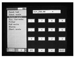
15. Using the up/down arrow keys select **Eng units** and touch **ENTER**. The alpha-numeric keypad will now be displayed allowing you to enter up to five characters to describe the engineering units for this particular point. There are multiple pages of text and symbols that can be used. Use the **PAGE**, **PAGEBK** and **SHIFT** keys to access different characters. For this example (0-250 psig) enter **PSIG** and touch **ENTER**.
