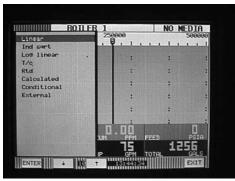
7. The menu displaying types of linear inputs should now appear. For this example use the up/down arrow keys to select **4-20 mA** and touch **ENTER**.
