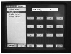
29. The 0-150 scale complete with EFFLUENT and GPM should be displayed on the Recorder. Use the VIEW button to select a particular display to verify your work. You will also notice that your high alarm set point is marked at 120 with an arrow.
