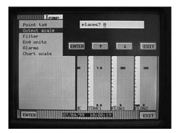
11. A numeric keypad will now be displayed prompting you with lo→ ←. This is where you enter the low end of your range or the equivalent value for 4 mA. For this example (0 to 150 gpm) select 0 and touch ENTER.
