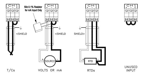
Figure 2-7 Thermocouple, RTD and Linear Inputs
