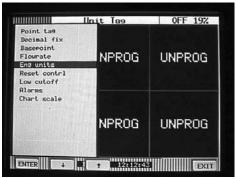
15. The alphanumeric keypad should now appear allowing you to enter up to 5 characters to describe the engineering units for this particular point. There are multiple pages of letters, numbers and symbols that can be used. Use the PAGE, PAGEBK and SHIFT keys to access different characters. For this example enter MG (for million gallons) and touch ENTER.
