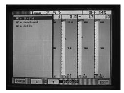
16. You will be prompted with alarm #?. Each point has 5 internal alarm set points. You can use the up/down arrow keys to scroll through 1, 2, 3, 4, or 5. Since this is the first alarm set point for channel one, select 1 and touch ENTER.
