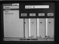
25. Use the up/down arrow keys to select **Scale ends** and touch **ENTER**. You will now be prompted with **places?**. Here you can select the number of decimal places that will be displayed on the virtual chart display. For this example use the up/down arrow keys to select **0** and touch **ENTER**.
