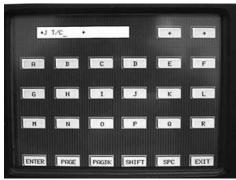
10. The menu starting with Point tag will again be displayed. Use the up/down arrow keys to select Decimal fix and touch ENTER. You will be prompted with places>? (0 or 1). Use the up/down arrows to select zero or one decimal place for thermocouples. For this example select 1 and touch ENTER.
