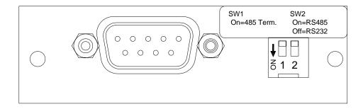
Figure 2-10 RS232/RS485 Modbus
