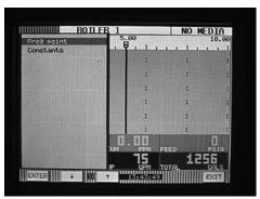
4. The numbers **1-9** and letters **A-F** represent the 15 channels that can be set up. Touch the number or letter that represents the input or channel you wish to configure. For this example use number **1** and touch **ENTER**.
