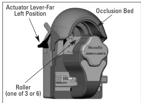
To unload tubing from the pump, turn off the drive. Then open the pump by moving the actuator lever counterclockwise (left), as described above. The pump will automatically open the tubing retainers, as well as lifting the occlusion bed away from the tubing. Then pull the tubing away from the pump front.
