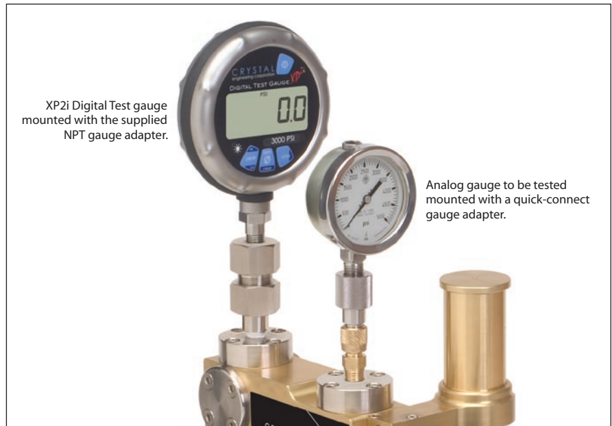
Figure 4. The GaugeCalXP Pressure Comparator can be configured with an XP2i digital test gauge and a gauge to be tested, in either of the two ports.
