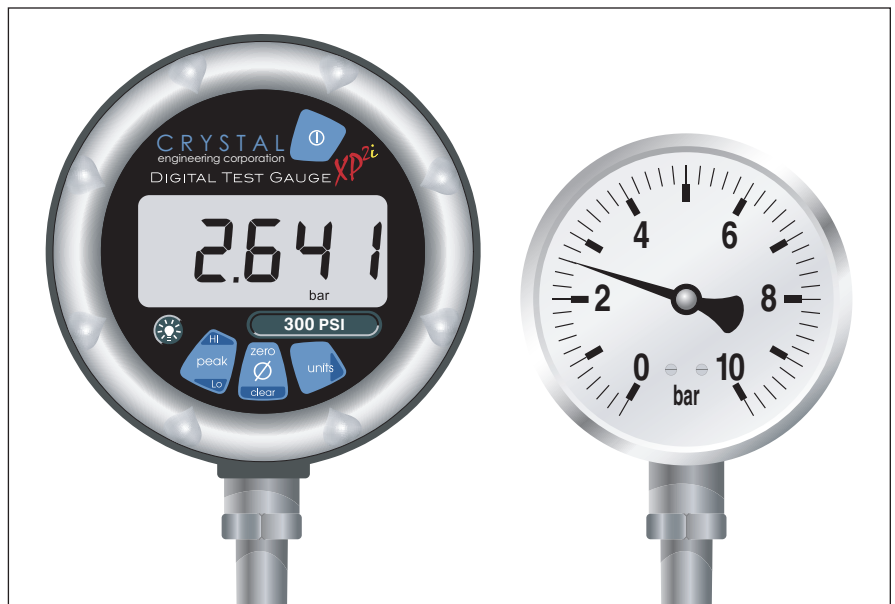
Figure 5. Checking the accuracy of an analog pressure gauge against the display of the XP2i digital pressure gauge.
