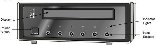
The Power button switches the interface on and off. It is disabled while measurements are being made.
