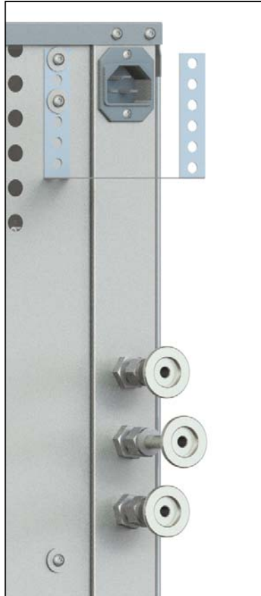
Fig. 15 Turn the tilt protection upwards
