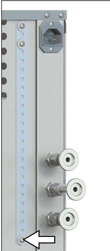
Fig. 14 Remove the screw right at the bottom from the tilt protection
