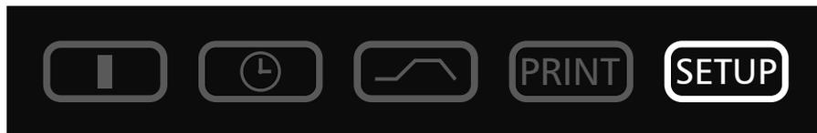
In this operating mode it is possible to make the basic settings of the oven. Clock time, date, day, year, and settings of sounder, of address assignment, monitoring units, heater power and calibration are set here.
