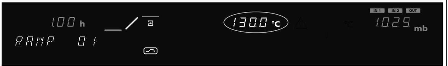
Setpoint temperature / temperature at the end of the ramp segment
