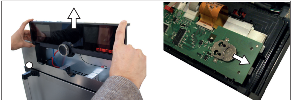
Fig. 38 Removing the lithium battery
