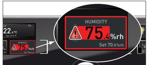
Fig. 22 Humidity monitoring triggered
