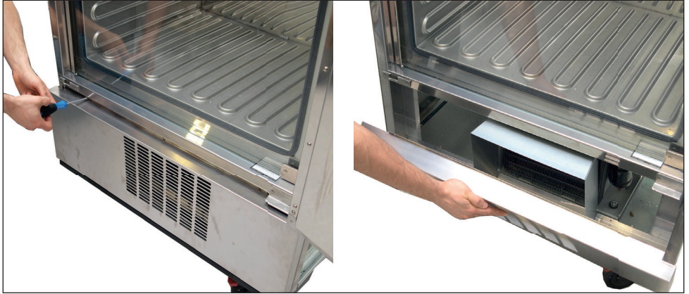
Fig. 30 Unscrew and remove the front cover
