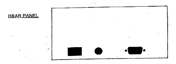
The rear panel shown above has the on/off power switch at the left, the 12 volt do power input jack in the middle and the RS232 I/O port on the right.
