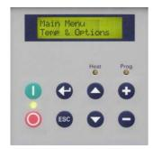
To control the system the controller has few "easy to use" buttons on a foil keypad. Simply press desired button.
