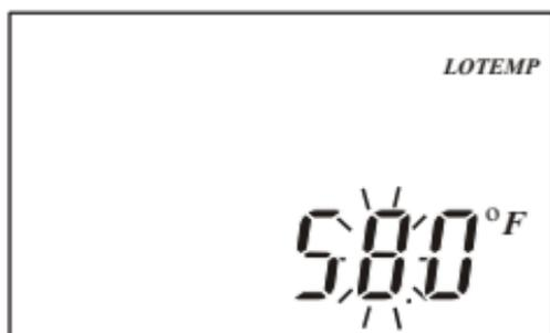
4. Press **PRG** key until it displays **SA**, release it, the display will show as Fig. 14 with **LOTEMP** flashing.
