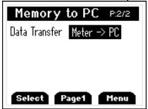
Once the USB connection is establish with PC, press the Select button to download data from Meter to PC using HyperTerminal.
