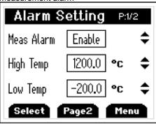
Disable or enable the alarm by pressing recall  $\blacktriangle$  or  $\log \blacktriangledown$  and F1 to accept. Increase or decrease individual limit by pressing recall  $\blacktriangle$  or  $\log \blacktriangledown$ .
