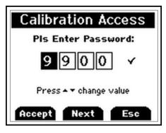
Before go into the calibration mode, must enter the password. Press F2 to change to the next digit. (Default Password is 9900) There are two calibration options:
