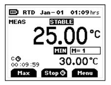
Press F2 key in the middle of a countdown will stop the process:
