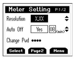
Press F1 to indicate you want to change the setting of the current parameter or recall  $\blacktriangle$  or  $\log \blacktriangledown$  to move to the next parameter.
