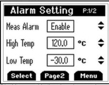
Disable or enable the alarm by pressing recall ▲ or log ▼ and F1 to accept. Increase or decrease individual limit by pressing recall ▲ or log ▼.
