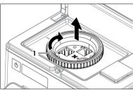
3 Lift the back cover (1) of the storage compartment.
