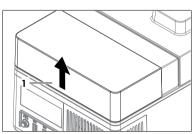
4 Lift the cuvette carousel out of the cuvette carousel bay.
