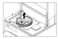
5 Hold the top of the cuvette containing second sample by the frosted sides (1) and lift it out of the rack.
