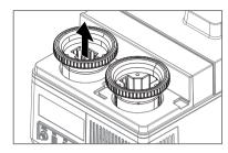
5 Insert the cuvette carousel (1) into the drip tray (2).
