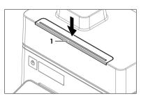
Slightly turn the cuvette carousel (1) and lift it out of the drip tray.
