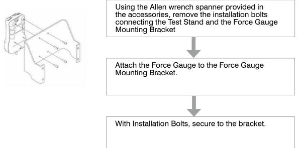
Attach the Force Gauge to the Mounting Bracket.
