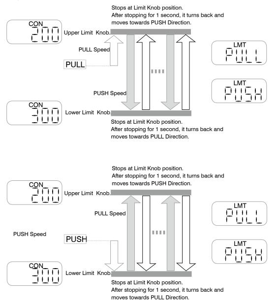
Change speed by UP, DOWN Key. SIg Mode and CON Mode Speed Setting are commonly used. During movement, speed variation is not possible. When no movement is occurring (at idle), the display shows movement Mode and the latest operated speed. When the movement starts, the respective memorized movement . Speed is displayed.
