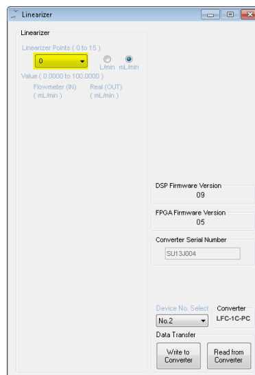
Figure 5: "Linearizer" menu of configuration software (Setting for no linearizer values)
