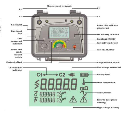
After starting a test the user will see confirmation of successful continuity testing on the LCD. If the dashes are not shown connecting 1 & 2 C and/or P leads connection has not been detected.
