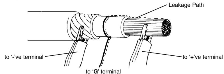
The guard terminal is at the same potential as the negative terminal. Since the leakage resistance is effectively in parallel with the resistance to be measured, the use of the guard causes the current flowing through surface leakage to be diverted from the measuring circuit. The instrument therefore reads the leakage of the insulator, ignoring leakage across its surface.
