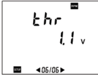
Figure 4-8 Display of the threshold voltage of the tachometer sensor.
