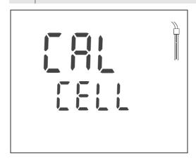
2 Press **<ENTER>** or **<CAL**\_\_> to confirm the selection of *CAL CELL*.
