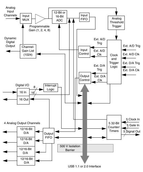
Figure 1 shows a block diagram of the DT9834 Series modules.
