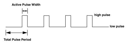
Figure 5: Example of a Low-to-High Pulse Output Type
