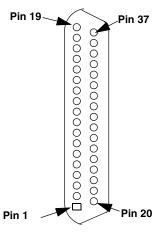
Figure 7: Orientation of the Analog Input Connector on the BNC Connection Box
