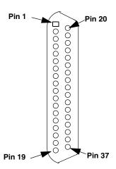
Figure 8: Orientation of the Digital I/O Connector on the BNC Connection Box
