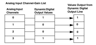
Figure 2: Example Using Dynamic Digital Outputs
