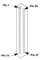
Figure 9: Orientation of the Analog Output, Counter/Timer, Clock, and Trigger Connector on the BNC Connection Box
