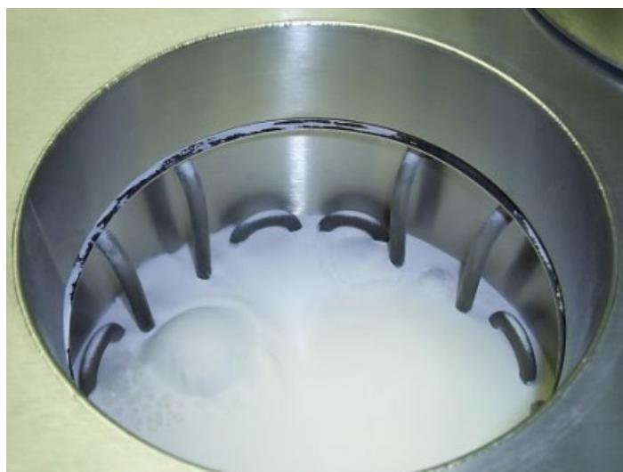
**Figure 3: Fluidized alumina at the correct operating level**
