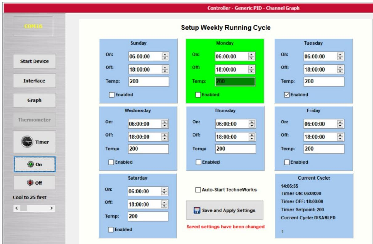
Setting up a bath start/stop sequence is fairly self-explanatory on this screen. Once the “On” time has been reached the bath will ramp up to the value set in the “Temp” window. At the “Off” time the bath will start cooling down to the setting in “Cool to value first”. After the “Cool to value first” is reached the bath will completely shut down and enter a sleep mode. The controller will display an FSH alarm when this occurs which is normal.
