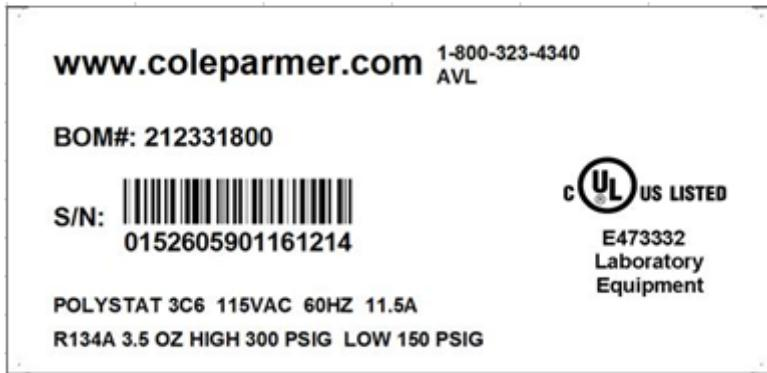
Use the nameplate on the rear to identify your immersion circulator/circulating bath, its electrical requirements and, if applicable, the refrigeration data. Cole Parmer catalog part numbers are listed in the specification tables in this section.
