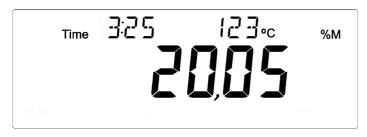
Showing a test in progress for 3:25 minutes, with a current temperature of 123°C and 20.05% moisture, the test is still running.
