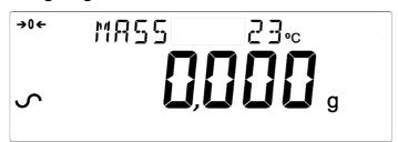
Showing no weight on the pan, stable and at zero point.
