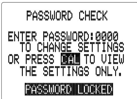
You will only see this page if the unit is password locked. To change any settings or calibration you need to unlock the system to remove the “**PASSWORD LOCKED**” message. You need to enter the correct 4-digit number on the “**ENTER PASSWORD**” input. You can still view all the pages of **Calibration/Setting mode** if the system is password locked by just pressing the [**CAL/VIEW**] key on this page. If the unit is “**PASSWORD LOCKED**” going to
