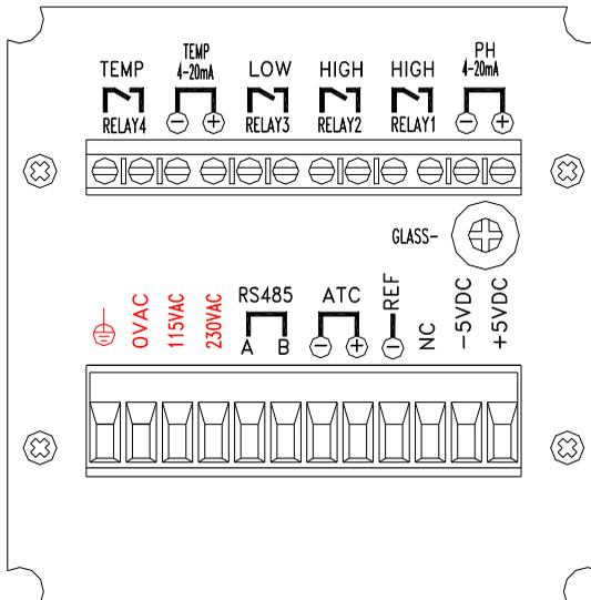
**CAUTION:** Make sure you connect the AC power cord to the correct AC terminals. Connecting incorrectly may damage the unit permanently.
