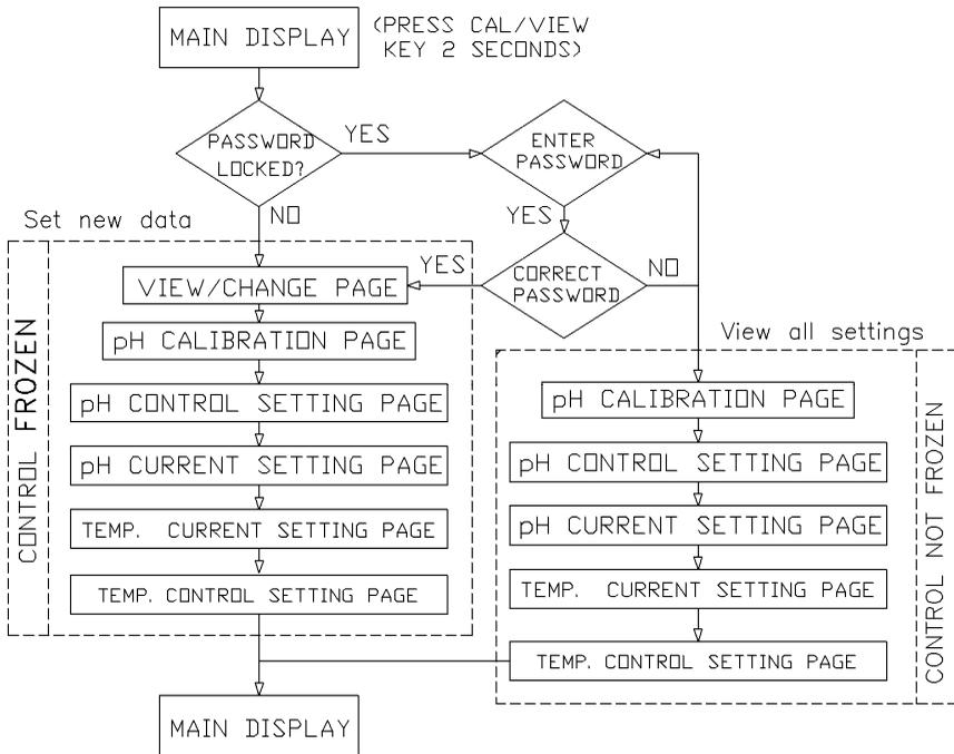
Pressing the [CAL/VIEW] key for about two seconds during main display mode will bring-up the first page of seven pages of the **Calibration/Setting** mode. Pressing [CAL/VIEW] key will switch to the next page until the last page, where pressing [CAL/VIEW] again will return the user to main display mode.
