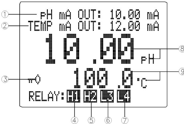
1. **pH mA OUT** - this will display the output of the pH 4- 20 mA circuit.
