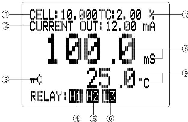
1. **CELL** – actual cell constant of the probe computed from the last cell constant calibration. In TDS display it will show the TDS factor instead of the cell constant.
