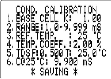
**1. BASE CELL K** – this is the basic probe cell constant. You can choose **0.01, 0.10, 1.0** or **10**. Be careful in changing this option since it will set the actual cell constant to this value and you must calibrate the cell constant before you can accurately use the unit.
