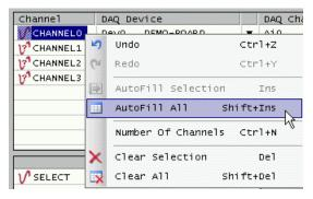
The dialog automatically becomes configured to acquire data from four channels on the DEMO-BOARD.
