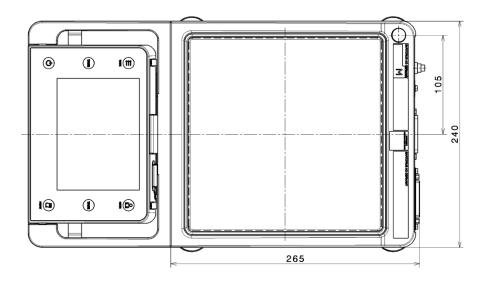
Precision Balances Without a Draft Shield (D0) (Toploader) – with MSE Display and Control Unit All dimensions are given in millimeters
