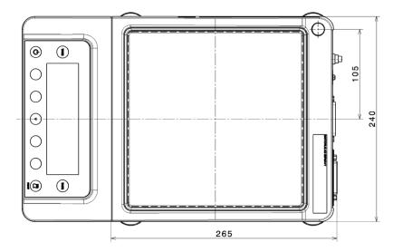
High-Capacity Precision Balances All dimensions are given in millimeters
