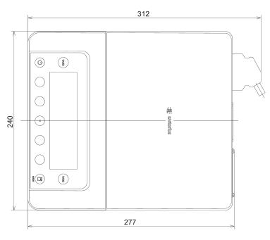
Ultra-Micro Balance | Micro Balance Weighing Module with DM Draft Shield All dimensions are given in millimeters
