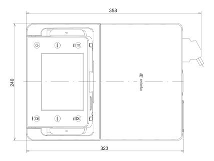
$\label{likelihood} \mbox{Ultra-Micro Balance} \ | \ \mbox{Micro Balance} \ - \ \mbox{with MSE Display and Control Unit and Electronics Module} \\ \mbox{All dimensions are given in millimeters}$
