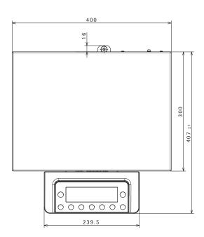
High-Capacity Precision Balances All dimensions are given in millimeters
