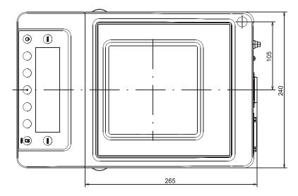
Precision Balances Without a Draft Shield (D0) (Toploader) – with MSA|MSU Display and Control Unit All dimensions are given in millimeters
