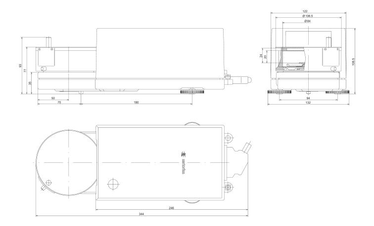
High-Capacity Micro Balances with DH Draft Shield All dimensions are given in millimeters
