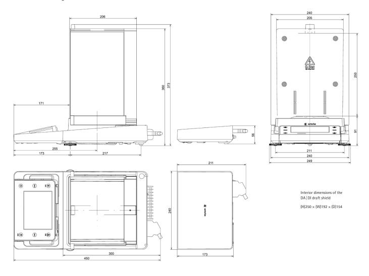
Semi-Micro Balances with Motorized Draft Shield – with MSE Display and Control Unit and Electronics Module All dimensions are given in millimeters
