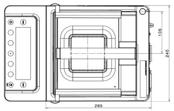
Interior dimensions of the DU draft shield (H)261 × (W)193 × (D)191 Precision Balances with a Readability of 1 mg or Model 5202S (with a Readability of 10 mg) and DE Draft Shield – with MSA|MSU Display and Control Unit
