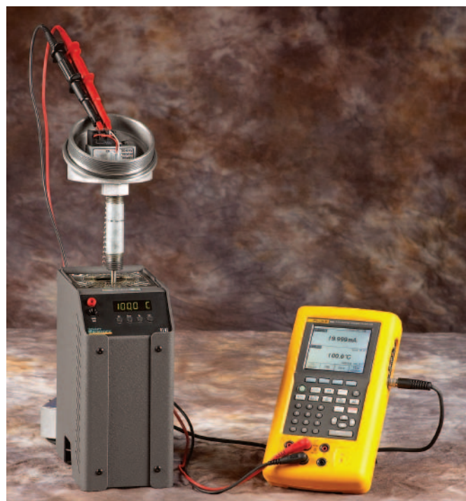
Figure 5. Fluke 744 and Hart Scientific calibrating a 4-20 mA transmitter and temperature sensor
