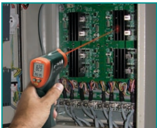
Max hold indicates and holds the peak temperature for easy identification of hot spots
