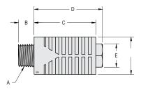
The 78165-50 and 78165-52 silencers have excellent noise reducing characteristics with minimal resistance to air flow. These silencers are one third smaller than comparable products, providing considerable space savings. The large surface of the felt element resists contamination far more than other materials such as sintered bronze, steel mesh or porous polyethylene.
