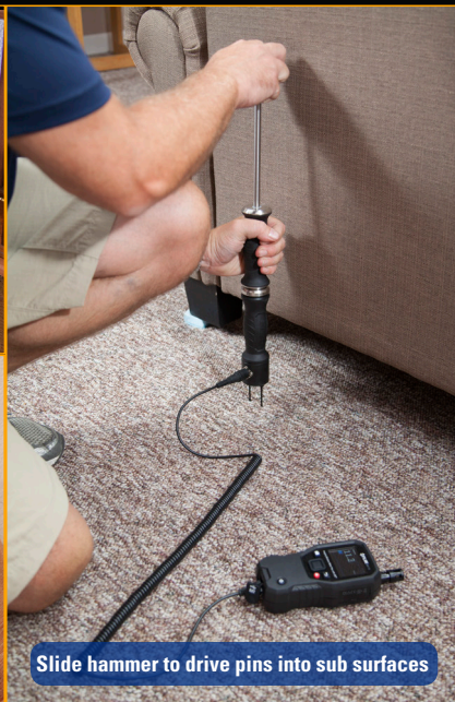
Probe up to 6" deep with the call cavity tool
