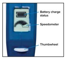
Turn thumbwheel and watch speedometer to fine-tune the speed.
