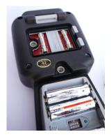
Separate battery and fuse access – Calibration Seal does not need to be broken for battery replacement.
