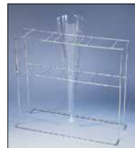
Imhoff settling cone shown with support rack
