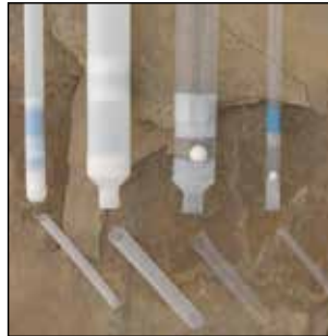
Polyethylene bailers are opaque; PVC and FEP bailers are clear.
