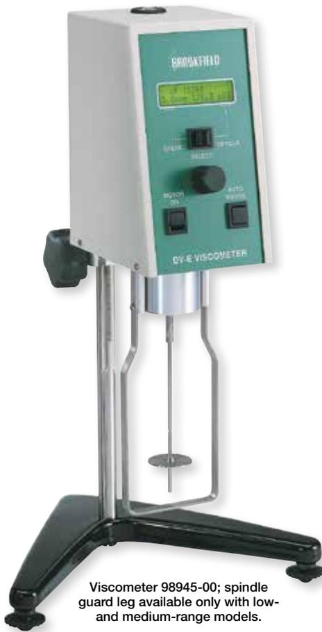
Viscometer 98945-00; spindle guard leg available only with low- and medium-range models.
