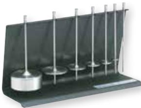
Spindle rack 98945-96; spindles not included
