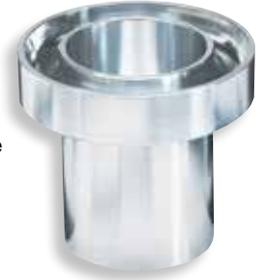
The cups are made from solid aluminum; the orifice is made from brass. All the cups are calibrated to NIST-traceable oils. NIST-traceable cups are available with an NIST-traceable calibration report supplied by the manufacturer. Cups conform to ASTM D333, D365, and D1200.
