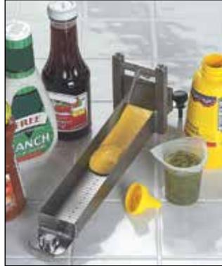
Consistometer requires only 75 mL of sample for measurement. Engraved graduations in 0.5-cm divisions ensure accurate results; spring-loaded gate prevents premature sample flow. Leveling screws and built-in spirit level help achieve repeatable results. Stainless steel construction prevents corrosion.
