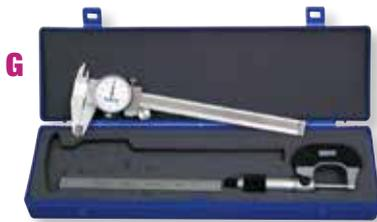
**G. Analog Measuring Kit** includes micrometer, caliper, flexible 6" rule, and carrying case. Micrometer reads 0 to 1"; 0.0001" graduations; accuracy is  $\pm 0.0001$ ". Features friction thimble, locking clamp, and carbide-tipped measuring faces. Caliper measures outside, inside, and depth to 0.100"; 0.001" divisions; accuracy is  $\pm 0.001$ ". Features thumbwheel and locking screw.
