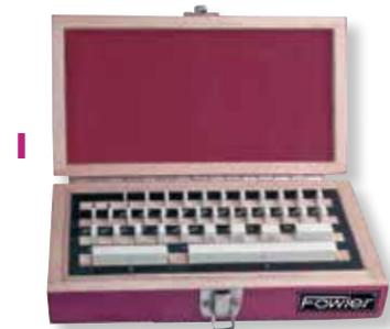
**I. Calibration Gauge Block Kits** are available in steel blocks that are abrasion- and corrosion-resistant. Block sizes range from 0.0625" to 2" (9-piece sets) and 0.10005" to 4.0" (36-piece set). Kits include a NIST-traceable calibration report supplied by the manufacturer and a protective wooden case.
