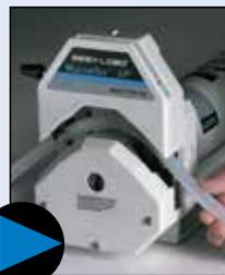
Move lever to the left to open pump head. Load the correct size tubing.
