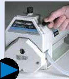
Rotate the lever to the right to close head. Adjust occlusion setting by turning knob on top of pump head.
