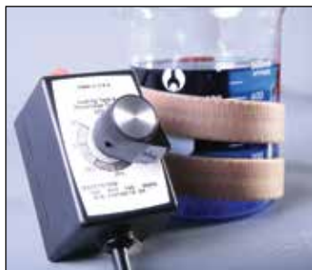
Time percentage controller regulates the time heater is on and off.
