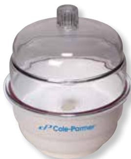
Desiccator has a chemical-resistant polypropylene (PP) body and polycarbonate (PC) cover. A neoprene O-ring offers a secure seal. Use grease on the flanges to make the unit completely airtight. Includes PP plate.
