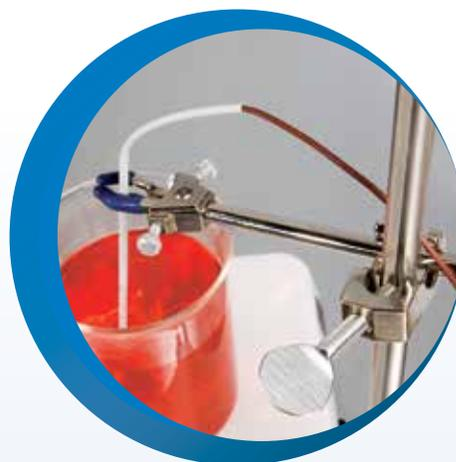
**External temperature probe kit**—includes 6" L probe, support rod, and clamp
